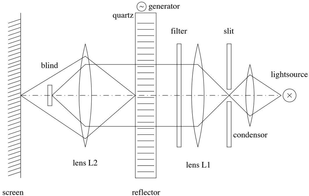
Figure 5: Schlieren method with two lenses
