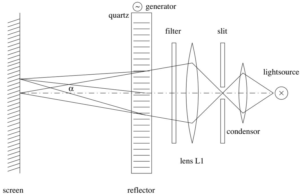
Figure 4: Diffraction method with one lens
