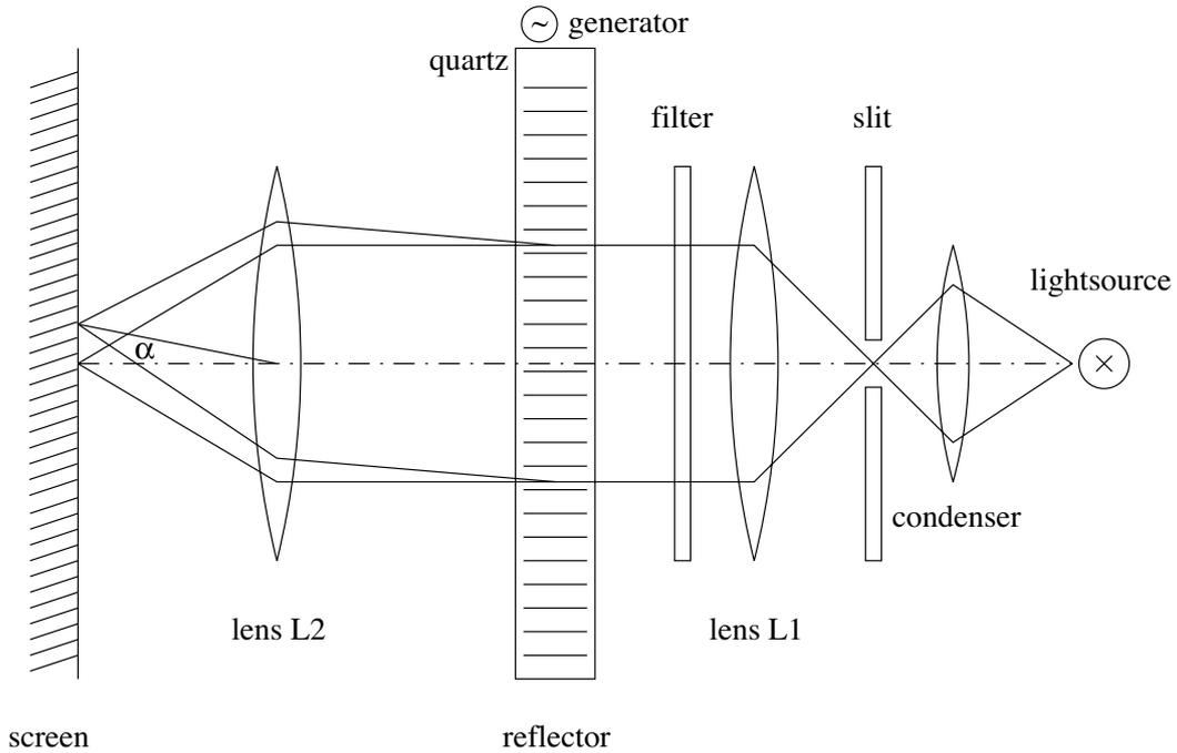
Figure 3: Diffraction method with two lenses
