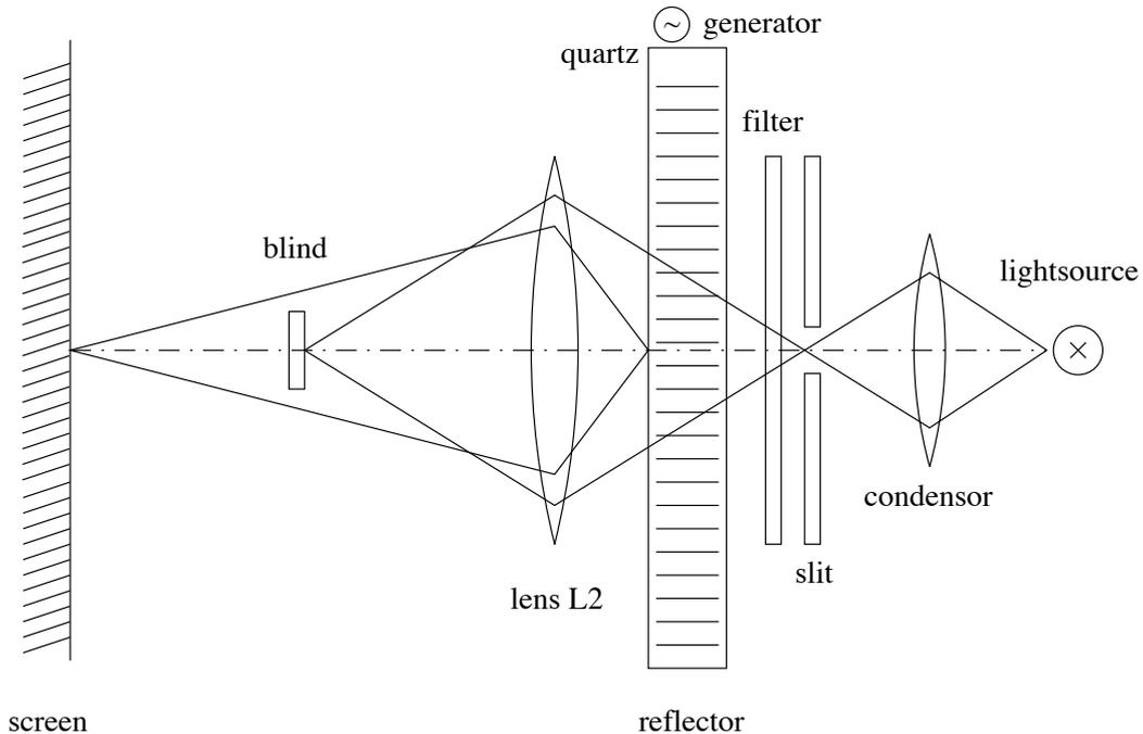
Figure 6: Schlieren method with one lens
