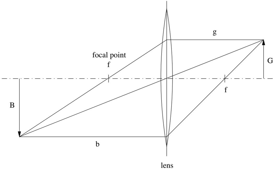
Figure 2: Construction of a picture projected by a collecting lens
