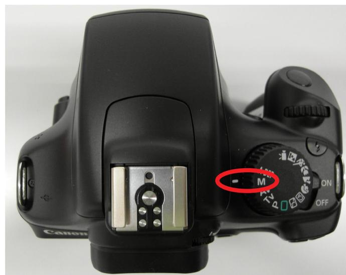
Figure 8: Setting the manual mode
